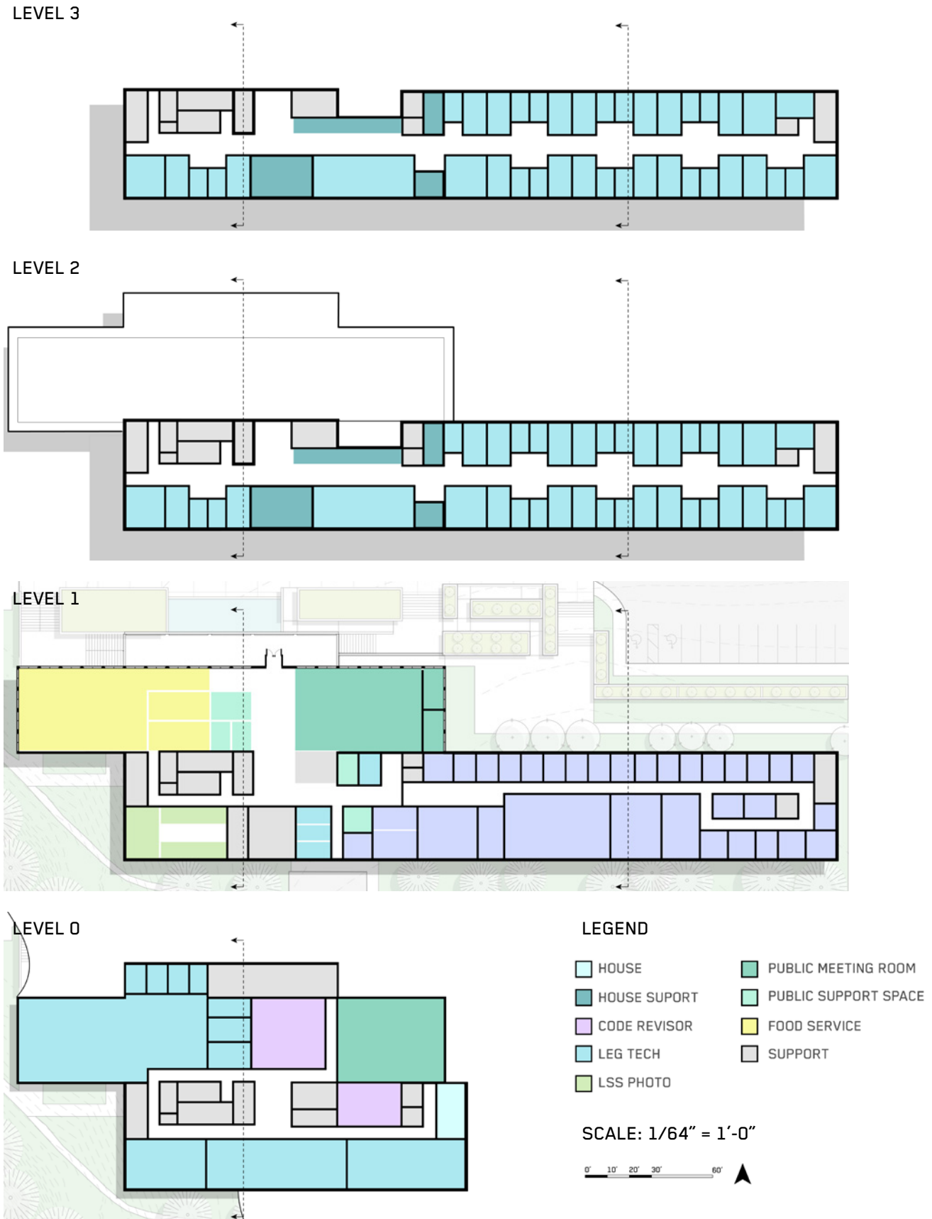
[FIGURE 15] PRITCHARD REHABILITATION/EXPANSION TEST-TO-FIT FLOOR PLANS
