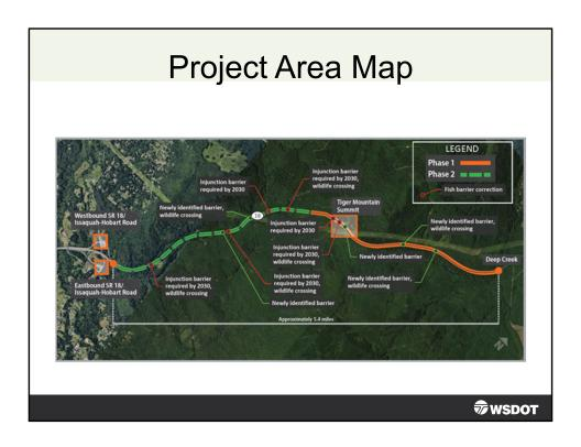
This slide provides the aerial map overview of the project area. The orange color depicts the elements for this project (phase 1). The green color is for future phase 2. Issaquah Hobart Road/SR18 Interchange is on the left side of the map. The two small squares represent the two roundabouts as part of this project. The next slide will provide the summary list of the scope.
