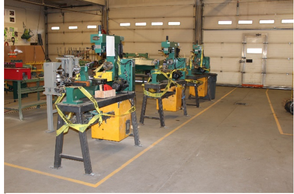
Mechanical areas have minimal circulation leading to safety concerns. Old bus garage doors can be seen in the background.
