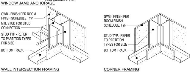
Interior - Typical Non-Load Bearing Metal Stud Partition Details
