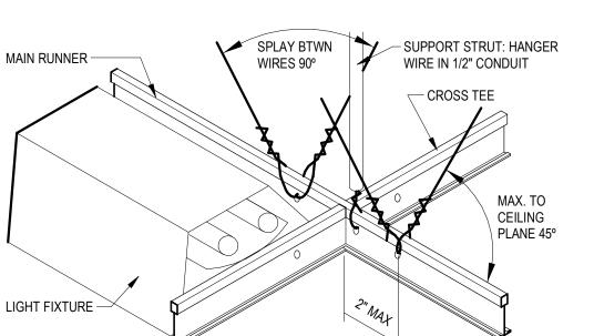
1. Provide grid & fixture installation in accordance with IBC 2506.2.1, ASTM C 635, Section 13.5.6 of ASCE 7 & UL fire resistance
