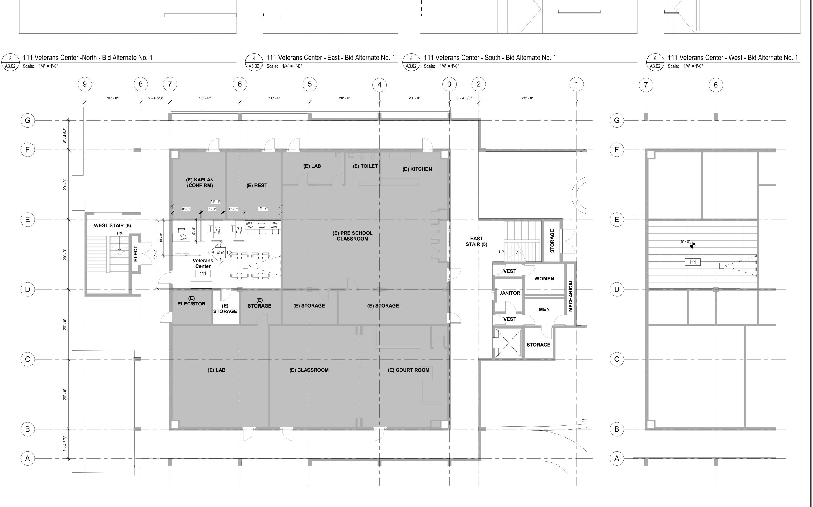
Level 1 - TI Floor Plan - Bid Alternate No. 1
