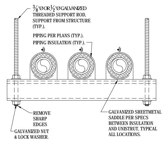
NOTE: PROVIDE THREE SUPPORT RODS FOR STRUT LONGER THAN 24"
