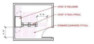
Figure 3: Typical Equipment Clearance
