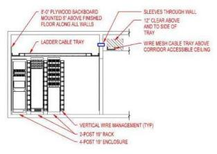
Figure 2: Example Section with Equipment
