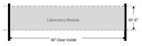
Figure M2 - Laboratory Planning Module
