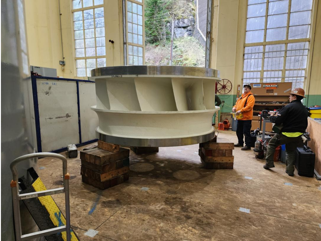
• Refurbished turbine runner
