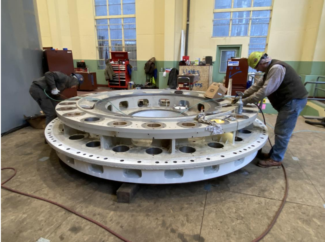
• Refurbished turbine Head Cover
