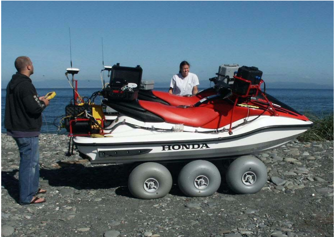
Figure 2. Second generation Coastal Profiling System being prepared for data collection.
