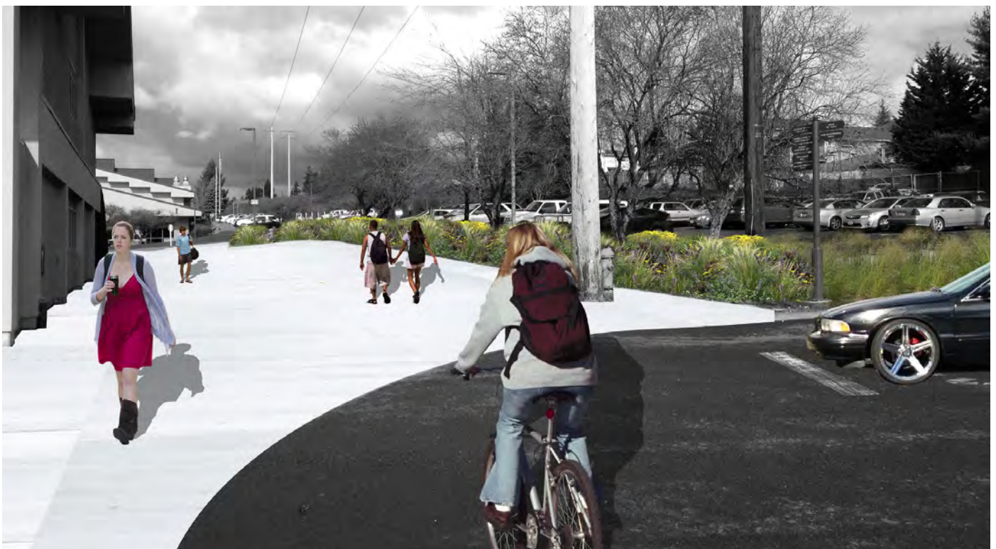
Rain gardens built into the parking islands near the staff parking lot will beautify this highly-public area while adding needed storm water detention capacity
