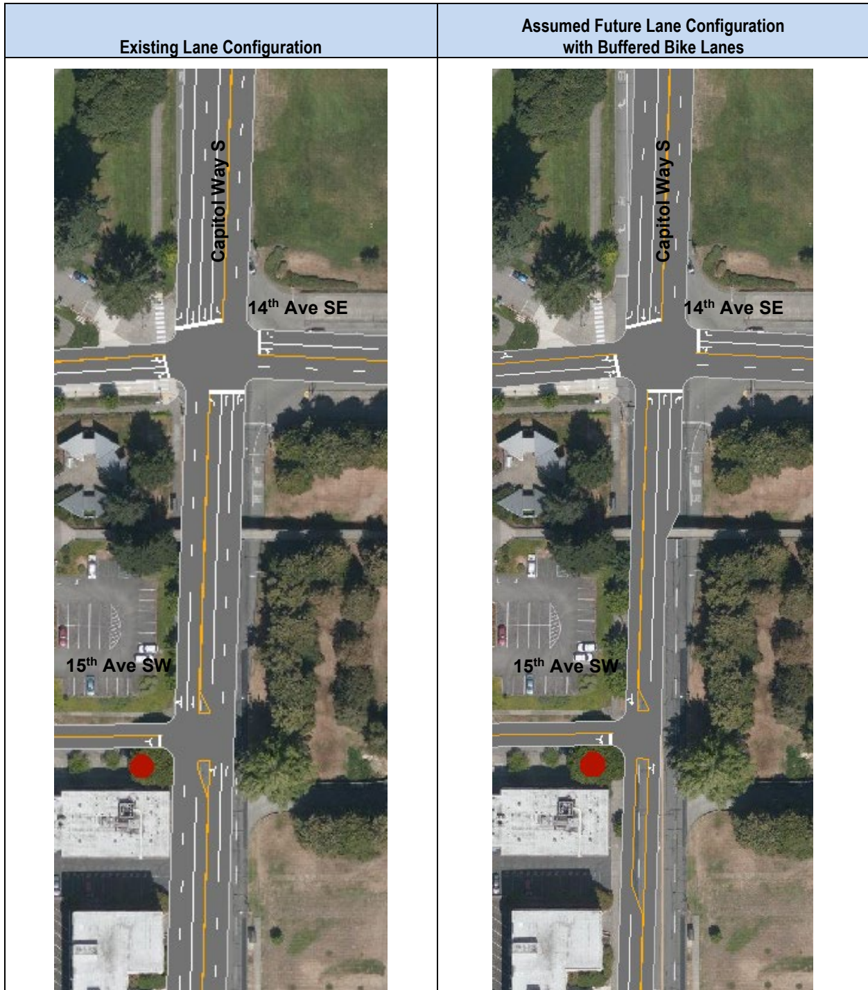
Figure 17. Existing and Assumed Future Geometry at Capitol Way S/14 th Ave SW Intersection
