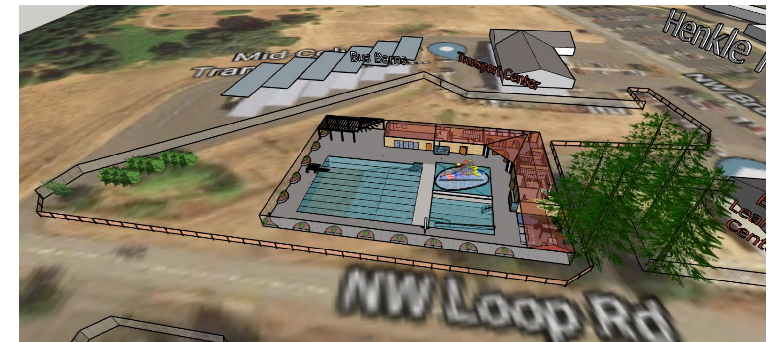
Indicative construction area perimeter fencing with the facility overlain for reference to proximity to school structures
