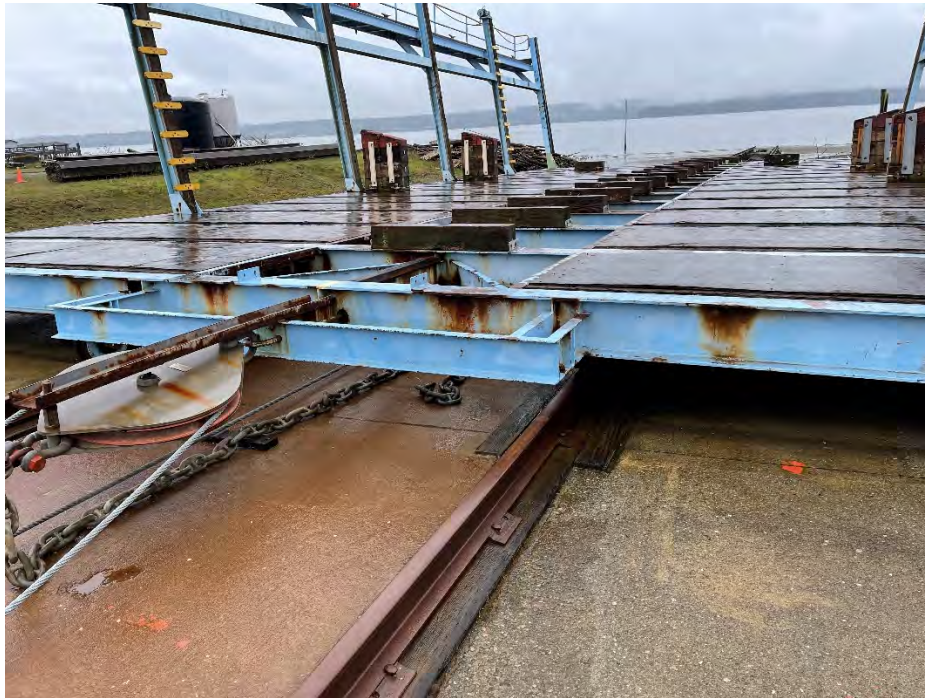
Photo 158: Cradle at Northern end of track
