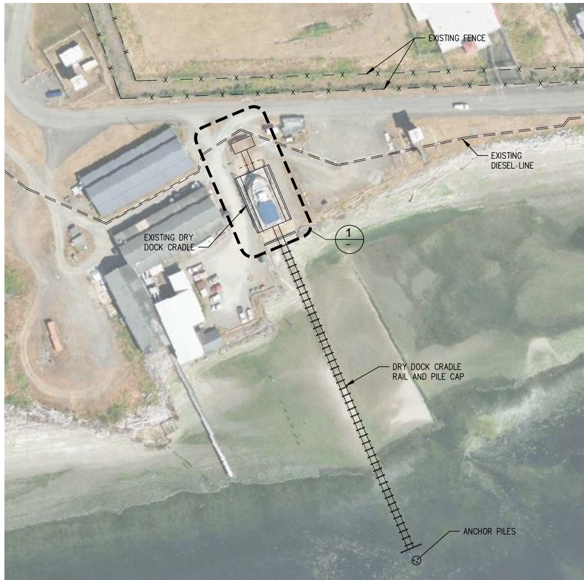
OVERALL EXISTING SITE PLAN SCALE: 1/64" = 1'-0"
