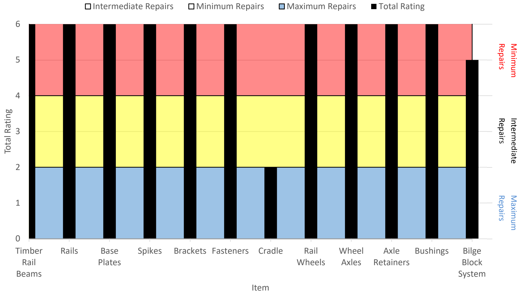
Figure 3. Total ratings with level of repairs for Railway Dry Dock miscellaneous items.
